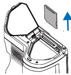
Next, insert and press the SD card deeper into its slot, until it clicks and then release the pressure. The card is now partially ejected and can be removed.
