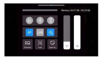
In the real-time image mode, click or slide up the icon at the bottom of the screen to pop up a shortcut menu. You may view the storage capacity of local memory or SD card and perform some quick operations, including brightness, volume, Bluetooth, Wi-Fi, laser, panoramic stitching, and super-resolution settings.
